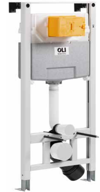
1200cm Pre-wall, freestanding w.c frame including brackets and w.c bend with 3/6 litre dual flush plate, front flush installation only.
